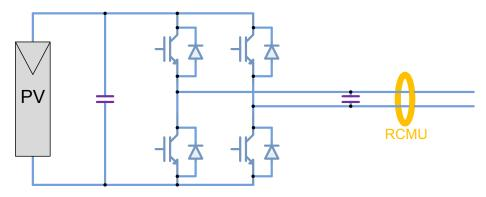
For no separation of power grid and the photovoltaic power generation between the inverter, according to VDE0126-1-1, there must be RCMU (residual current monitoring unit).
